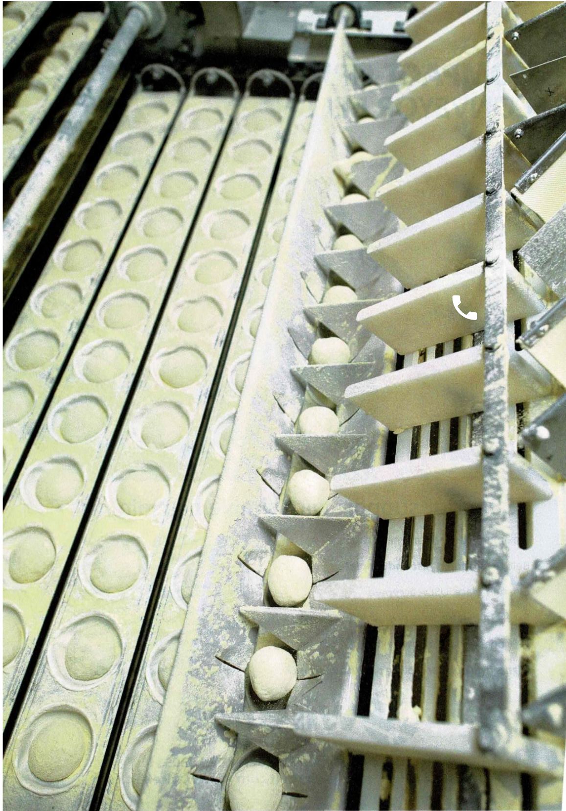
Figure 5 – dough balls at end of zigzag board in staging cup to be placed into the mesh basket for proofing. [3]
