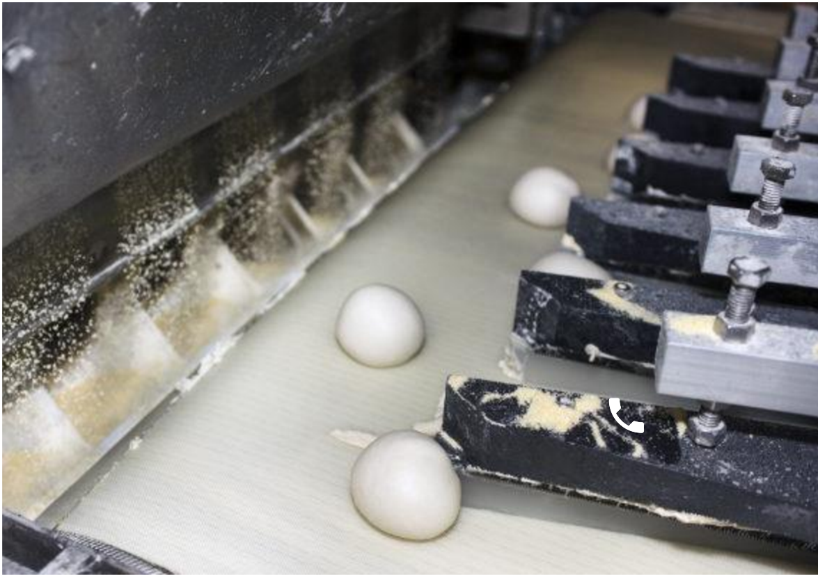
Figure 3 – end of molder and before zigzag board with dusting [6]
