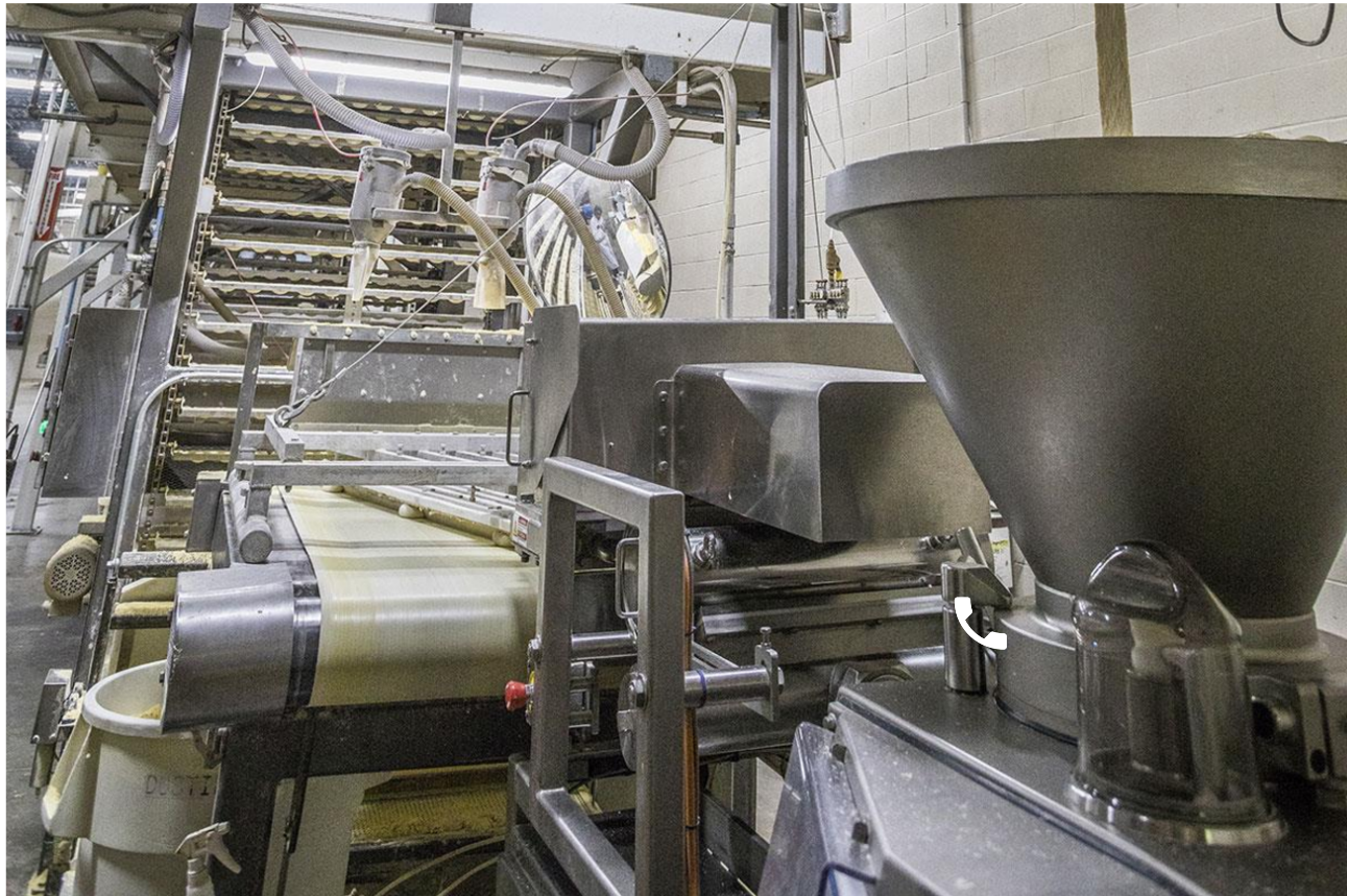
Figure 2 – dough divider, rounder dusting [not seen], and carrier taking muffin baskets up to the overhead proofer [front to back of photo [4]]
