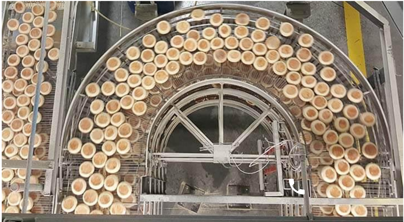
Figure 8 – muffin cooling conveyor [5]
