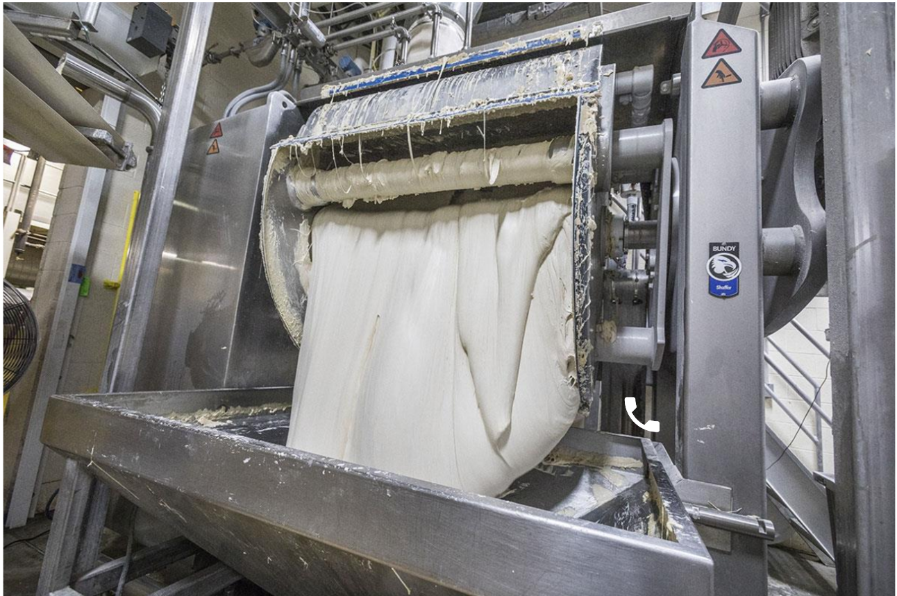
Figure 1 – dough exiting mixer - New Horizon [4]
