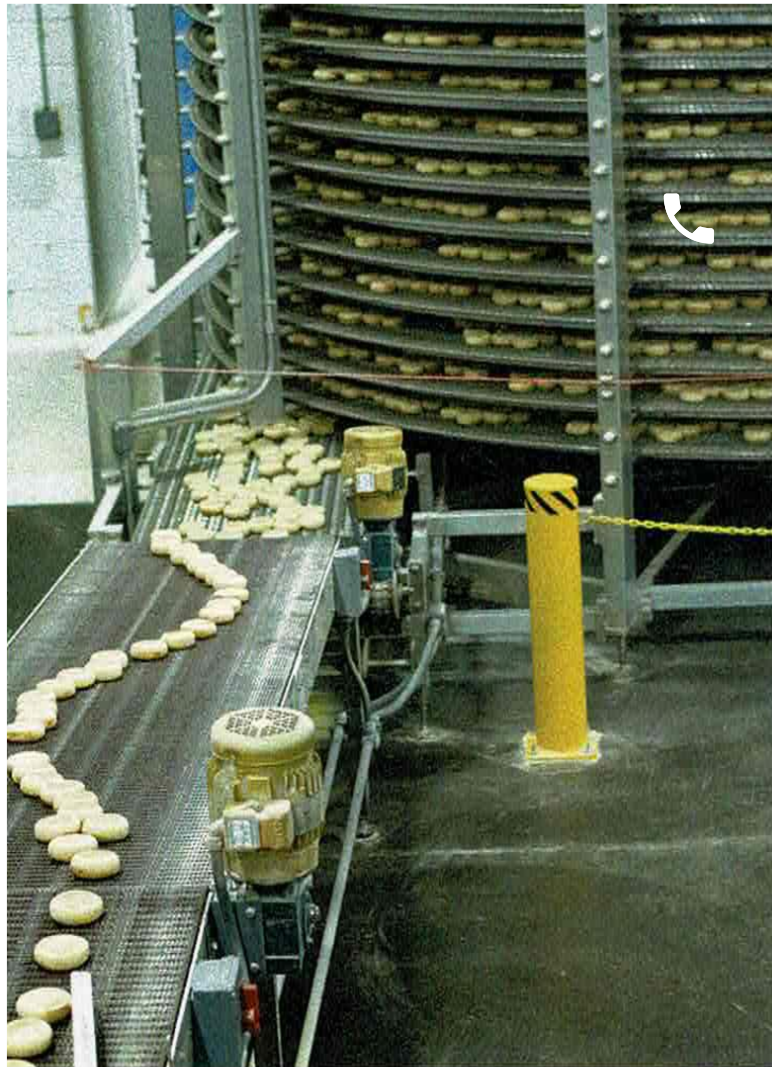
Figure 7 – Exiting oven and entering the cooling tower [5]
